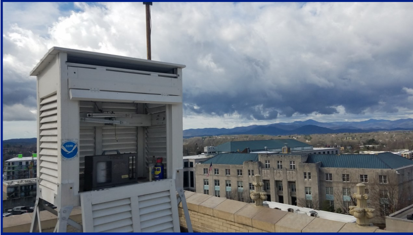
A Cotton Region Shelter (CRS) containing maximum and minimum thermometers at the NWS Cooperative Station atop The Grove Arcade, Asheville, NC.
