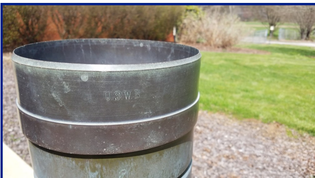
A vintage 8-inch Non-Recording Standard Precipitation Gauge, the standard for precipitation measurements for over 100 years within the NWS Cooperative Observing Program.
