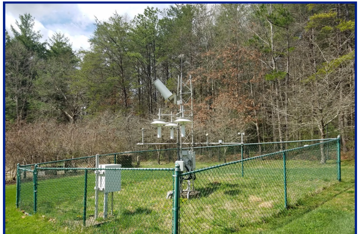
U.S. Climate Reference Network (USCRN) site located at the NC Arboretum (Buncombe County NC). A climate monitoring system that uses high-quality instruments which measure temperature, precipitation, wind speed, soil conditions and more. This data is used to monitor climate trends and are used to support ongoing climate research. There are 100 of these sites nationwide.
